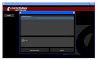
Select (click) the appropriate device. Then click <connect> if the device doesn't connect automatically. A notice will appear confirming connection to the AURORA light unit.
