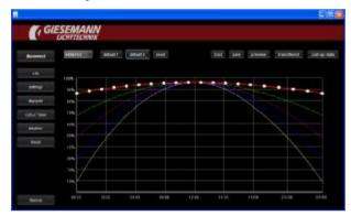
The chart starts on the left of the horizontal axis at 00:00hrs running to 23:59hrs on the right. The five color channels with their respective light intensities and durations are shown as time/intensity curves (0 - 100%) with intensity shown on the left of the graph on the vertical axis.
