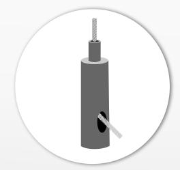
Mount the ceiling fasteners with suitable screws and dowels. Screws and dowels are not included in the scope of delivery, since different conditions always require individual mounting components. When mounting, make sure that the masonry # on site provides sufficient support.
