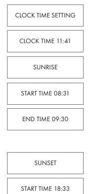
Open this menu with the Enter key <del>4</del> to set the lighting times for the fluorescent tubes.
